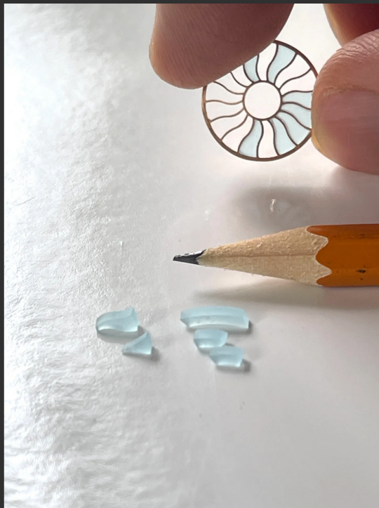
Cutting stones to size and working them into the intricate filigree of the Ulysse Aqua dial
